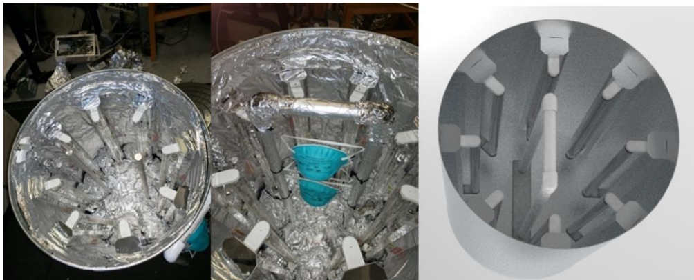
Fig. 4. Cylindrical design chamber. The chamber can hold up to 4 masks in the central support frame.
