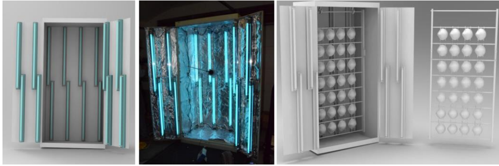
Fig. 3. Vertical cabinet with two front doors. The cabinet is a standard metal storage cabinet approximately 2 m high which was chosen to provide sufficient height to accommodate an upper and lower bank of UV-C lamps. The upper and lower banks are offset to fit into the cabinet and have a small region of overlap which does not appear to materially impact the vertical intensity profile in the cabinet. The CAD model illustrates a supporting frame containing 28 masks in 7 rows of 4. We estimate up to 40 masks could be loaded per UV-C exposure procedure in this design.
