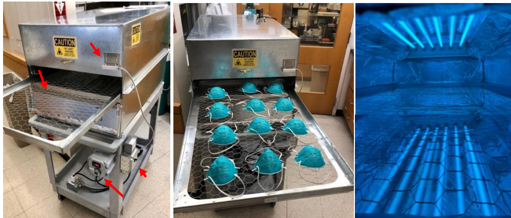
Fig. 2. Horizontal UV-C-decontamination chamber. The masks rest on a horizontal metal mesh support. A thin wire mesh (1-inch hexagon) was chosen as a tray to allow UV-C exposure on both sides while minimizing interference due to shadowing.
